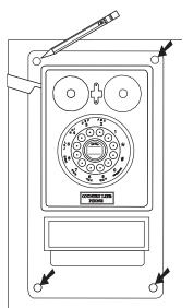
2. Tape the paper "template" on the wall at the desired mounting location.
